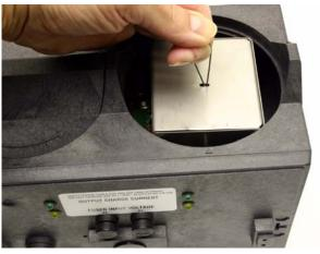
Figure 5-4 Inserting an SLA2191EX Battery Pack into the Charger
